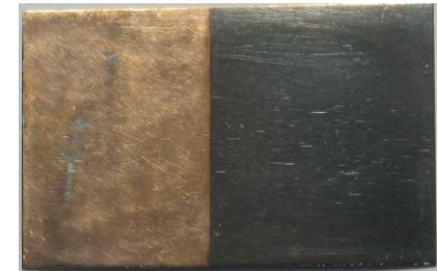
Copper coated with 200 nm of Tribo-Xt
