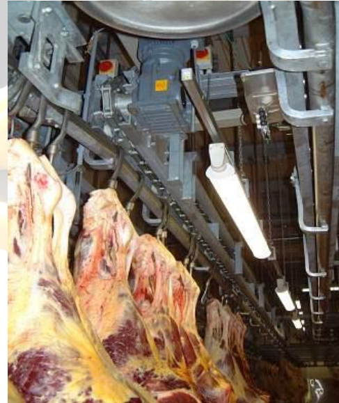
Conveyor Chain and Gearbox above the foodstuff
