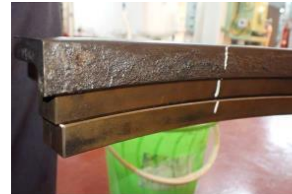
Piston Ring Backsides showing low deposit buildup
