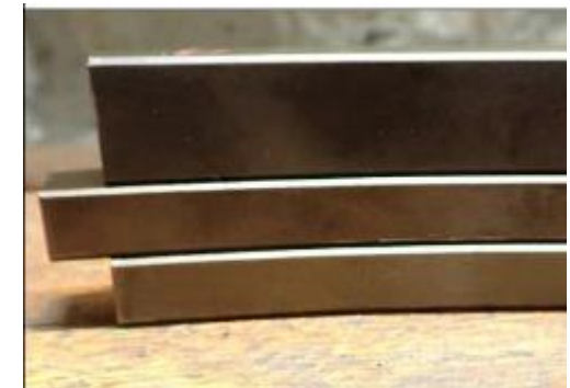
Piston Ring Backsides showing no deposit buildup
