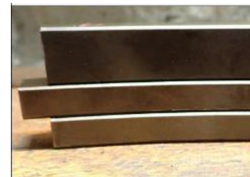
Piston Ring Backsides showing no deposit buildup
