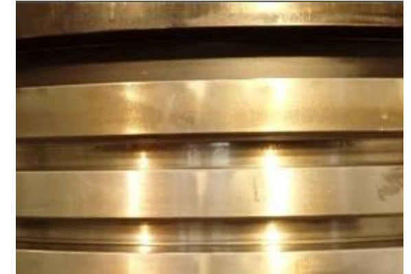
Piston Crown as removed showing ring grooves
