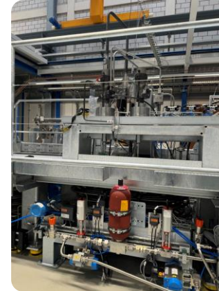
X52DF-A injector and injection system at the hydraulic rig in ERIC (Switzerland)
